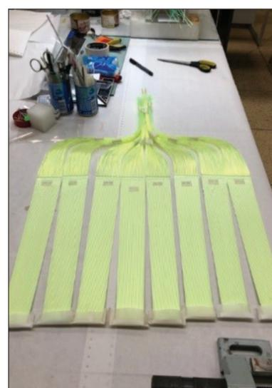
Left: ASTRA-M detector at the FSD spectrometer. Right: External view of individual elements of the ASTRA-M detector. The element is a (Ag)/<sup>6</sup>LiF scintillator plate, which is shaped like a time-focusing surface with glued wave-length-shifting fibers that transmit the light flux from the neutron capture site to the photomultiplier
