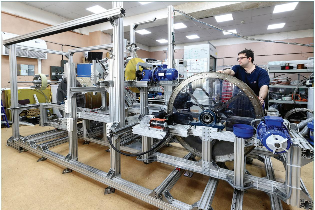
Installation of the HTS magnets winding
