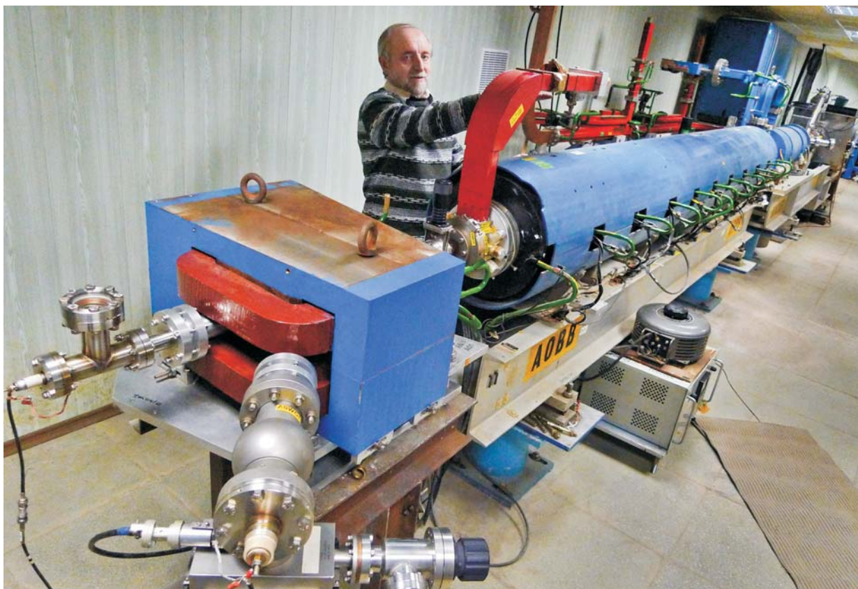
Dzheleпов Laboratory of Nuclear Problems. The first accelerating section of the electron accelerator LINAC-800
