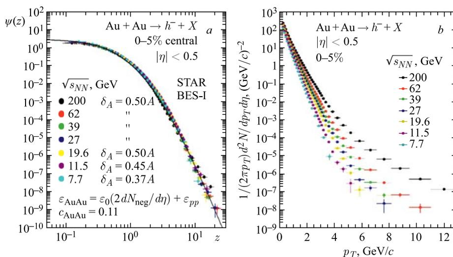
Fig. 2. The dependence of the scaling function  $\psi(z)$  (a) on the self-similarity parameter  $z$  for the corresponding momentum spectra (b) of negatively charged particles produced in the central Au + Au collisions at energy  $\sqrt{s_{NN}} = 7.7$ –200 GeV in the range  $|\eta| < 0.5$  [6]
