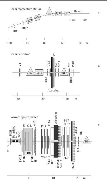
Fig. 4. The scheme of the Beam Momentum Station and the Beam Definition Station at the end of the CERN muon beam M2 and the SMC spectrometer
