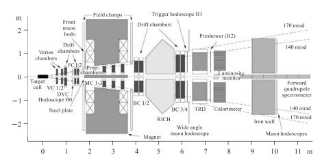
Fig. 5. A scheme of the HERMES spectrometer (side view)
