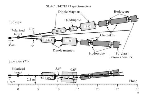
Fig. 6. Layout of the 4.5 and 7° spectrometers used in the E142 and E143 experiments
