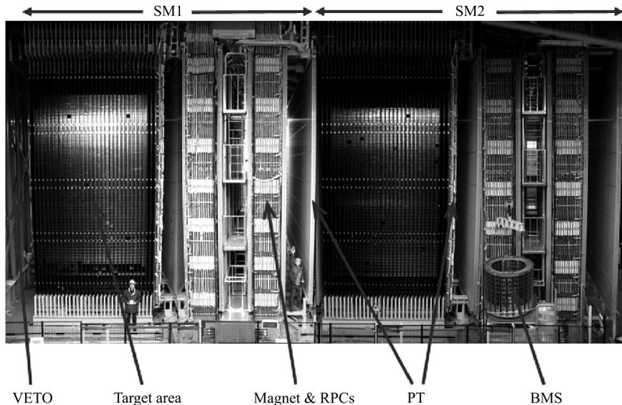
Fig. 1. View of the OPERA detector. The neutrino beam enters from the left. Arrows show the position of the VETO planes, the target and TT, the drift tubes (PT), the magnets and the resistive plates chambers (RPC) installed between the magnet iron slabs
