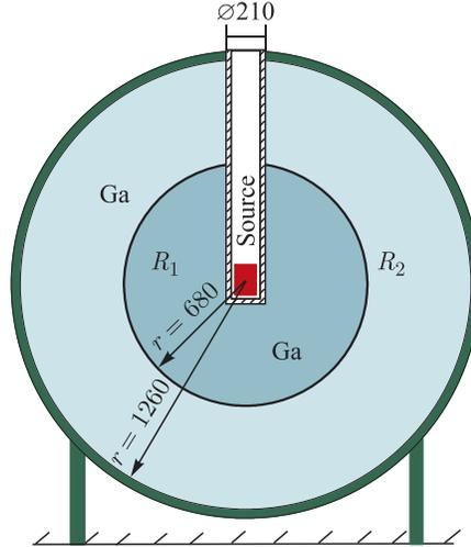
Fig. 2. Schematic drawing of the proposed experiment.  $R_1$  and  $R_2$  are the ratios of measured capture rate to predicted rate in the inner and outer zones, respectively. Outer radii  $r$  of the two zones and diameter of source re-entrant tube are given in mm
