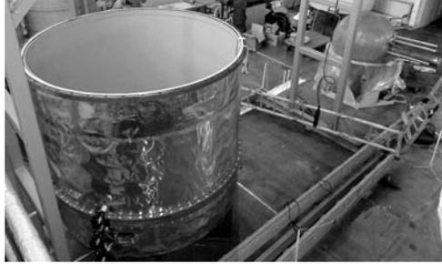
Fig. 8. The outer tank is completely prepared for the installation of the inner sphere
