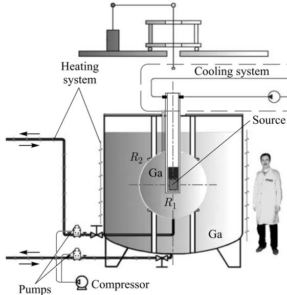
Fig. 4. Layout of the 2-zone facility
