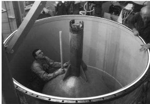
Fig. 9. The inner sphere is placed into the outer cylinder
