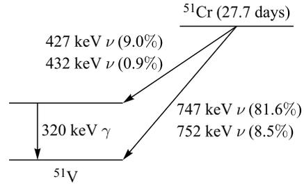
Fig. 3. Decay scheme of  $^{51}\text{Cr}$  to  $^{51}\text{V}$  through electron capture
