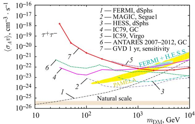
Fig. 4. Upper limits and sensitivities on DM annihilation cross section in tau-lepton channel from NTs and gamma-ray telescopes (see the text)
