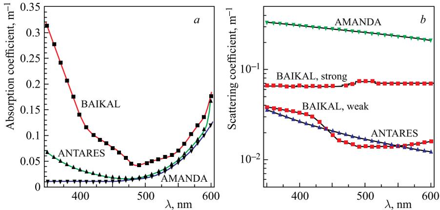
Fig. 1. Spectral dependence of absorption (a) and scattering (b) coefficients of the Baikal water, the Mediterranean Sea water, and Antarctic ice (from [7])
