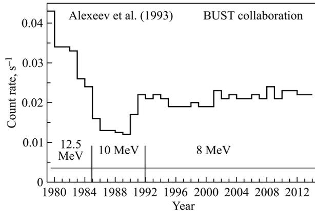
Fig. 2. The mean count rate of single events in three telescope internal planes (1200 counters) vs. the counter operation threshold
