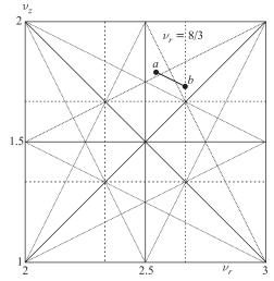
Fig. 8. The USR betatron tune diagram. Shown are: a — operation point of circulating beam  $\nu_r = 2.5443$  and  $\nu_z = 1.7905$ ; b — excited resonance  $\nu_r = 2.6637$  and  $\nu_z = 1.7315$  in the process of slow extraction. Also shown are I, II, III, IV operation points of original USR design [2]
