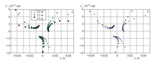
Fig. 10. Resonance extraction separatrices at the position of the electrostatic septum: *a*) different sextupole location at 12 m (triangles), at 23 m (stars) and at 33 m (squares); *b*) adjusting of separatrix arm orientation by simultaneous powering of two sextupoles  $k_{\text{Sx}} = -6 \text{ m}^{-2}$  at 12 m and  $k_{\text{Sx}} = +1 \text{ m}^{-2}$  at 23 m (stars) as well as  $k_{\text{Sx}} = +1 \text{ m}^{-2}$  at 12 m and  $k_{\text{Sx}} = -6 \text{ m}^{-2}$  at 23 m (circles)
