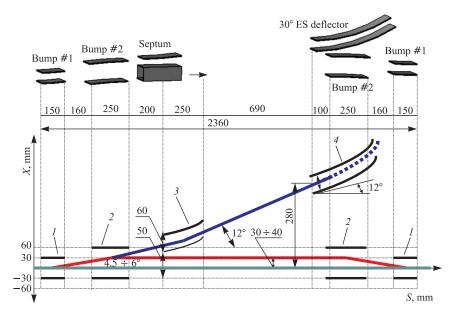
Fig. 2. Location of elements of the combined extraction systems in one of the USR straight sections: I — parallel plate bump electrodes #1; 2 — parallel plate bump electrodes #2; 3 — 6° electrostatic septum deflector of cylindrical shape, entrance tilt angle to the axis is variable from 0 to 6°; 4 — 30° electrostatic deflector
