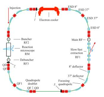
Fig. 1. Modified layout of the USR. Extraction section is outlined. Possible locations of sextupole for slow extraction: I -at 12 m; 2 -at 23 m; 3 -at 33 m
