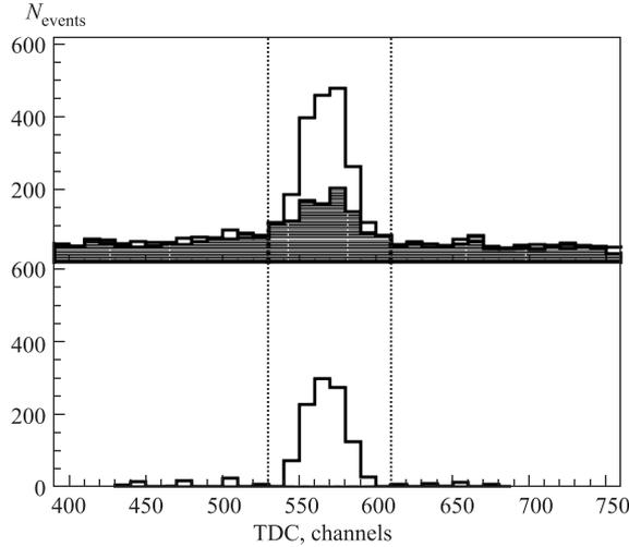
Fig. 7. Time difference distribution for  $dp$ -elastic events obtained from  $\text{CH}_2$ -C subtraction at a deuteron energy of 2.0 GeV
