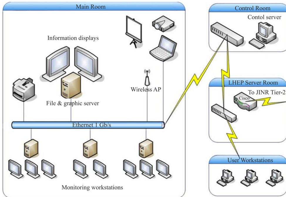
Fig. 2. The scheme of the JINR Remote Operations Center
