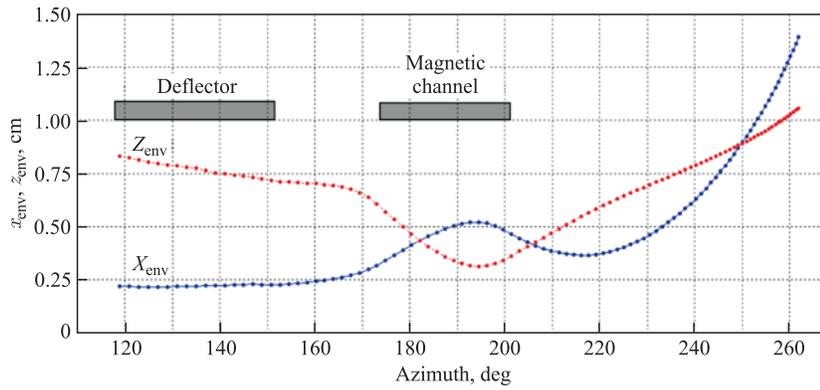
Fig. 18. RMS values ( $2\sigma$ ) of the beam envelopes
