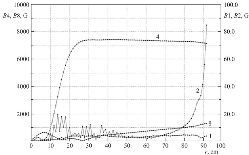
Fig. 5. Measured harmonics of magnetic field versus radius
