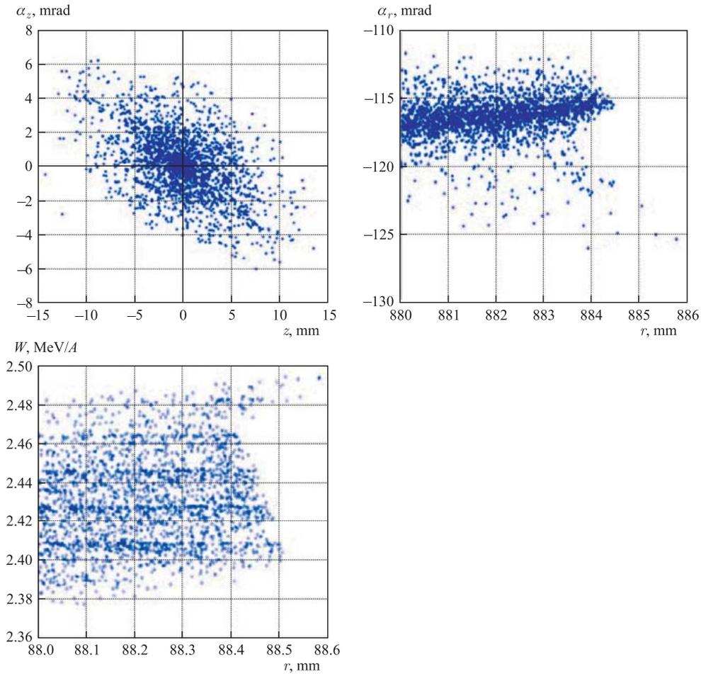
Fig. 15. Parameters of 2150 ions at the entrance of the deflector
