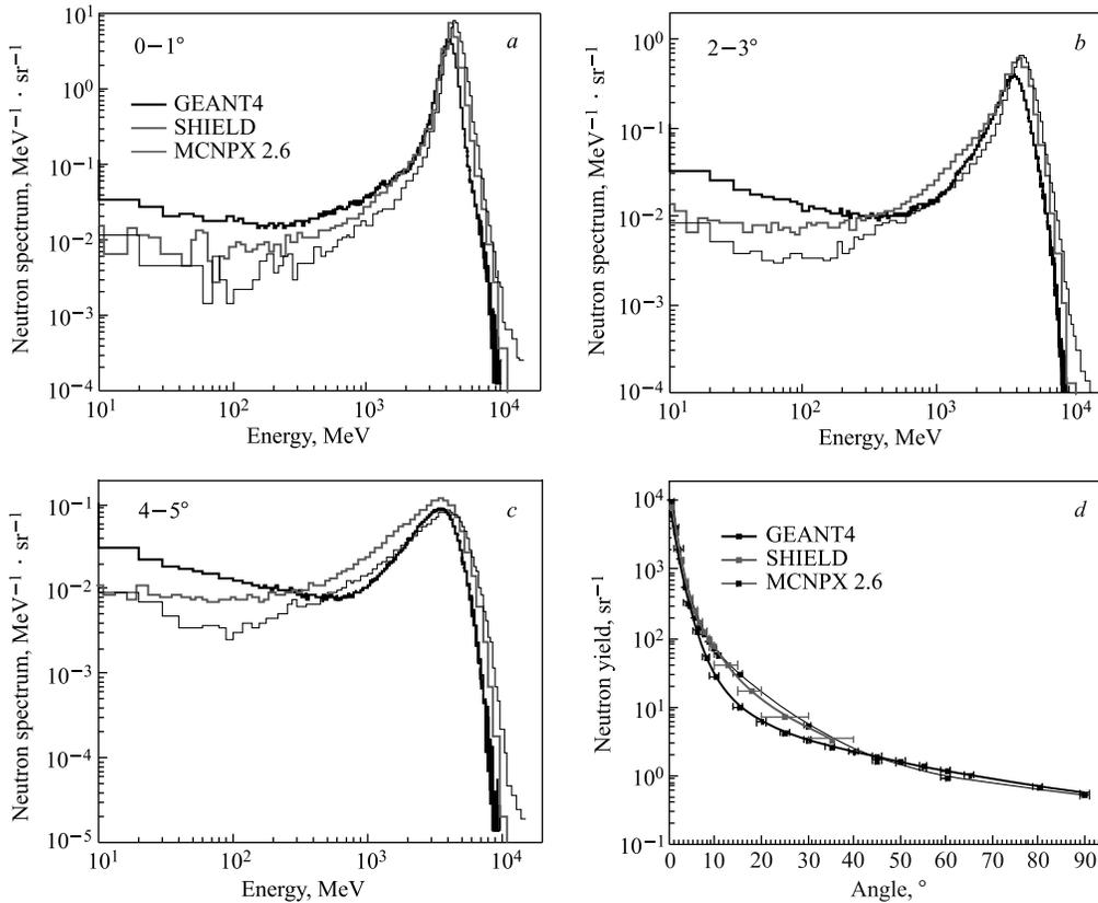
Fig. 1. *a–c*) A comparison of the secondary neutron spectra for the reactions  $^{197}\text{Au}(4.5 \text{ GeV/nucleon}) + {}^{\text{nat}}\text{Fe}$  simulated by the GEANT4, SHIELD, and MCNPX 2.6 codes. *d*) A comparison of the angular distributions of neutrons for the reactions  $^{197}\text{Au}(4.5 \text{ GeV/nucleon}) + {}^{\text{nat}}\text{Fe}$
