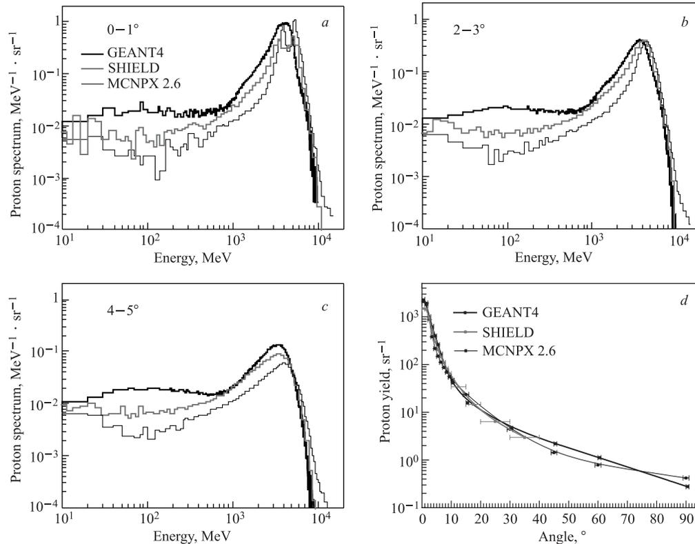
Fig. 2. *a–c*) A comparison of the secondary proton spectra for the reactions  $^{197}\text{Au}(4.5 \text{ GeV/nucleon}) + ^{\text{nat}}\text{Fe}$  simulated by the GEANT4, SHIELD, and MCNPX 2.6 codes. *d*) A comparison of the angular distributions of protons for the reactions  $^{197}\text{Au}(4.5 \text{ GeV/nucleon}) + ^{\text{nat}}\text{Fe}$
