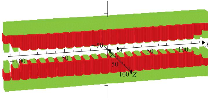
Fig. 4. TOSCA 3D simulation of the THz wiggler
