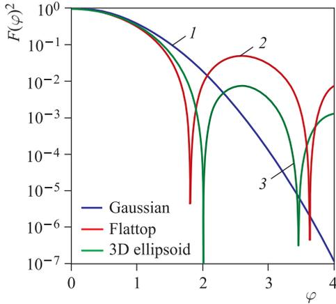
Fig. 2 (color online). Dependence of the squared form factor for the Gaussian (blue, 1), flattop (red, 2) and ellipsoidal (green, 3) beams on  $\varphi = \omega\sigma_z/c$
