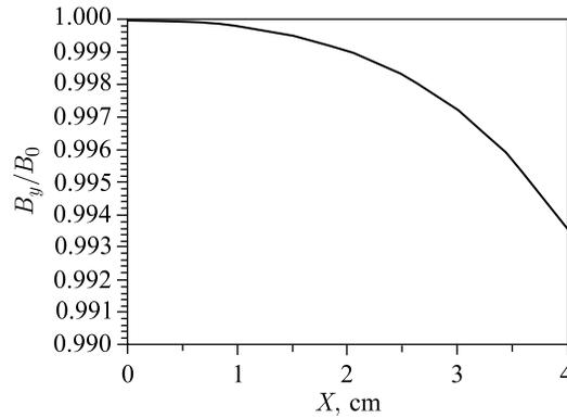
Fig. 6. Dependence of the normalized wiggler magnetic field at  $I_w = 21.5$  kA · turns on the transverse coordinate
