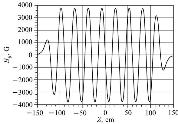
Fig. 5. Dependence of the wiggler magnetic field on longitudinal coordinate
