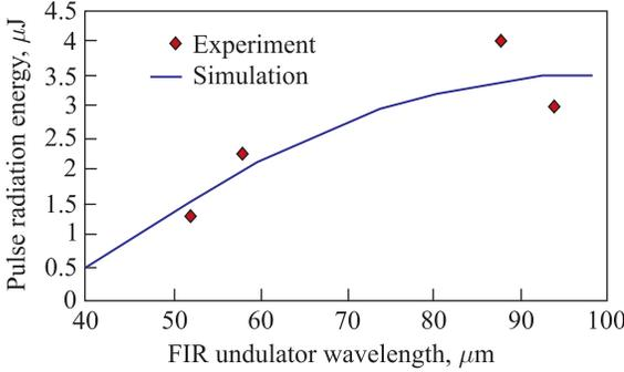
Fig. 1. Dependence of the FIR undulator pulse radiation energy on the wavelength
