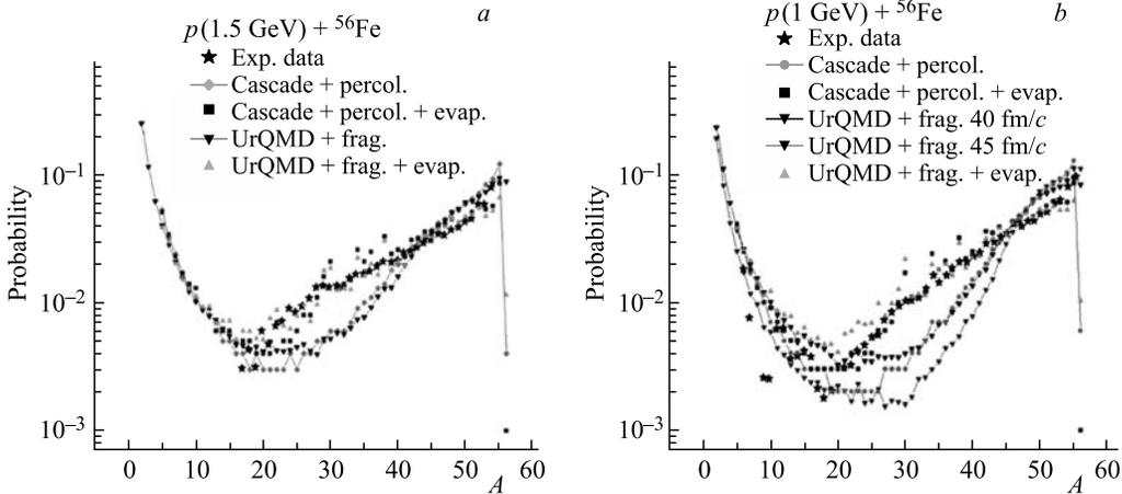
Fig. 2. Mass distributions of fragments in  $p + \text{Fe}$  for different proton energies: a) 1.5 GeV; b) 1.0 GeV [10]
