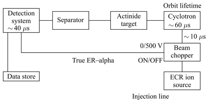
Fig. 1. Block diagram of the real-time process
