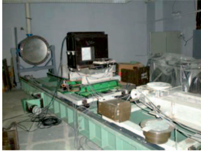
Fig. 6. PSD in shielding installed on the 8th channel
