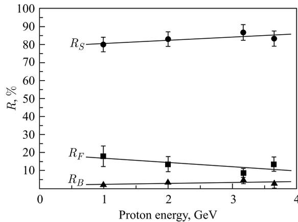
Fig. 6. Dependence of relative fission reaction yields on the side ( $R_S$ ), front ( $R_F$ ) and back ( $R_B$ ) surfaces on proton energy: the points — the experimental data; the curves — the linear fits
