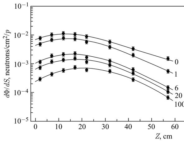
Fig. 1. Neutron distributions over the side surface of lead target obtained for a proton energy of 0.99 GeV: the points — the experimental data; the curves — the polynomial fits; the numbers — the minimal neutron energy in MeV
