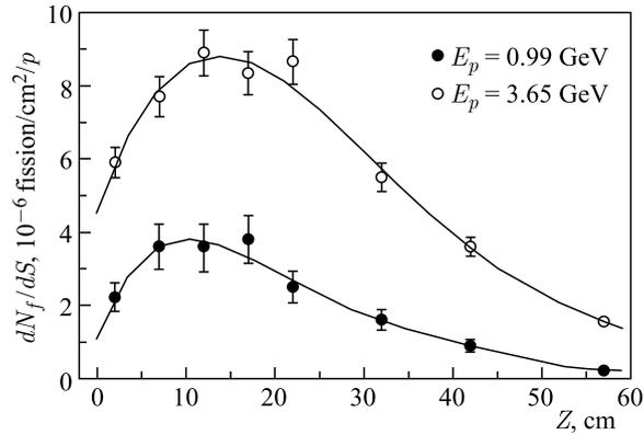
Fig. 5. Distributions of fission reaction rates of  $^{232}\text{Th}$  in  $1\text{-g/cm}^2$  layer over the side surface of target for two proton energies of 0.99 and 3.65 GeV: the points — the experimental data; the curves — the polynomial fits
