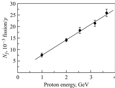
Fig. 8. Total fission reaction rate of <sup>232</sup>Th in 1-g/cm<sup>2</sup> spherical layer around the lead target: the points — the experimental data; the curve — the linear fit
