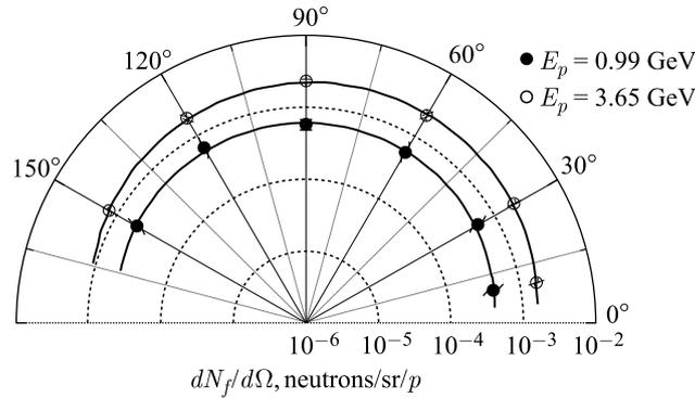
Fig. 7. Angular distributions of thorium fission reaction rate measured with 0.99- and 3.65-GeV protons for thorium layer 1 g/cm<sup>2</sup>: the points — the experimental data; the curves — the polynomial fits
