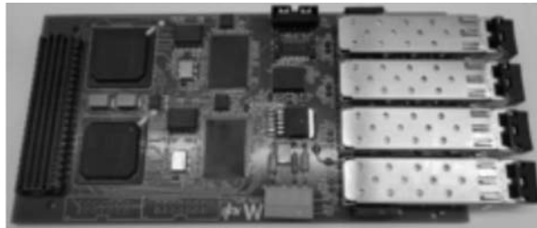
Fig. 2. The FTK Input Mezzanine Cards, four of which attach to the Data Formatter through the FMC connector
