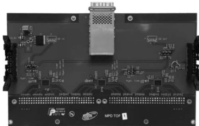
Fig. 1. 24-ch NINO based front-end board with Molex's CXP connector as an output
