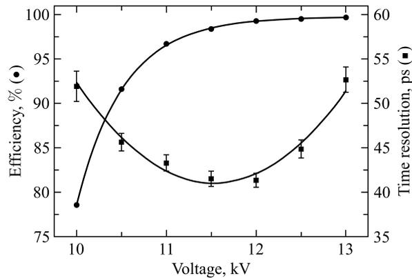
Fig. 4. Voltage dependence of the time resolution and efficiency
