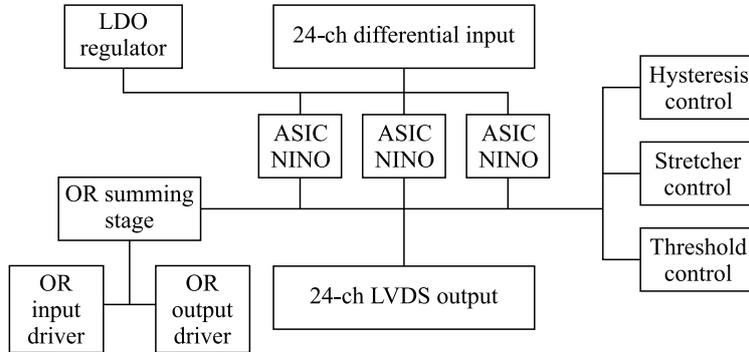
Fig. 2. Block diagram of the TOF preamplifier board based on the NINO chips
