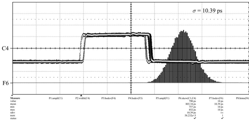
Fig. 3. Time distribution between two FEE board channels
