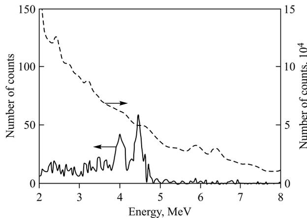
Fig. 7. Complete gamma spectrum (on the right) and a fragment of the spectrum (on the left) selected via discrimination of the background by the tagged-neutron technology
