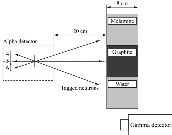
Fig. 5. Vertical layout of containers
