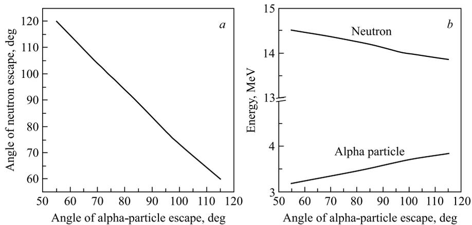
Fig. 2. Angle of neutron emission (a) and energies of a neutron and alpha particle (b) as functions of the exit angle of the alpha particle
