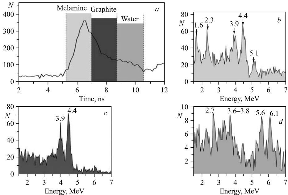
Fig. 4. Time spectrum (a) and gamma spectra corresponding to the time of passage of the containers with melamine (b), carbon (c), and water (d) by tagged neutrons for horizontal layout of containers
