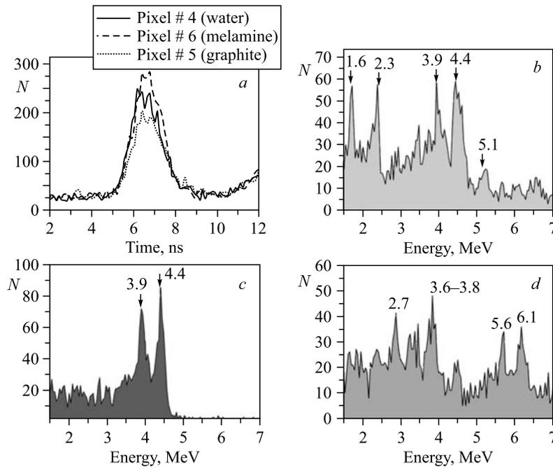
Fig. 6. Time spectrum (a), and gamma spectra corresponding to the time of passage of the containers with melamine (b), carbon (c), and water (d) by tagged neutrons for vertical layout of containers
