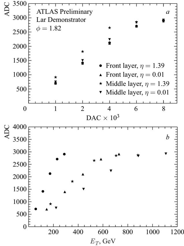
Fig. 14. Pulse maximum in ADC counts for four different super cells from the demonstrator for injected calibration pulses amplitude in DAC (a) and transverse energy (b) [5]
