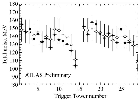
Fig. 10. The total noise in the trigger readout path on the demonstrator system in transverse energy in MeV. Trigger Tower 1–14 correspond to 0 to 1.4 in  $\eta$  and 16–29 are the same in  $\eta$ , but adjacent in  $\phi$ . The values represented by the full circles were measured by a spectrum analyzer, and the values shown in open circles were measured with Flash ADCs [5]
