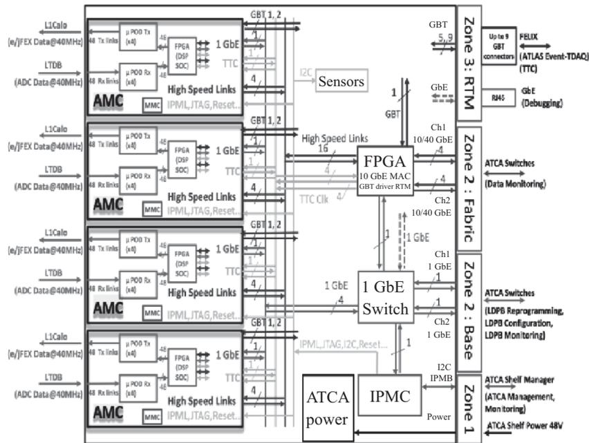
Fig. 4. Schematic diagram of LDPB, which contains four AMCs (see Fig. 5)
