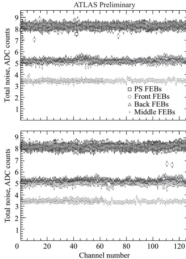
Fig. 8. The RMS of pedestal run for channels of the Front-End Boards in the demonstrator crate (a) and same sets in the neighboring crate (b). There are 28 Front-End Boards per crate, each has 128 channels. The noise levels of the boards vary because different capacitances and gains are applied to their respective cells [5]
