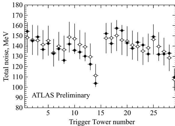
Fig. 10. The total noise in the trigger readout path on the demonstrator system in transverse energy in MeV. Trigger Tower 1–14 correspond to 0 to 1.4 in  $\eta$  and 16–29 are the same in  $\eta$ , but adjacent in  $\phi$ . The values represented by the full circles were measured by a spectrum analyzer, and the values shown in open circles were measured with Flash ADCs [5]
