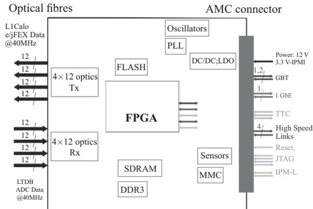
Fig. 5. Schematic diagram of an AMC, with an ALTERA Arria-10 FPGA in the center
