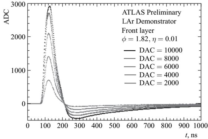
Fig. 13. Pulse shapes of a super cell from the demonstrator for injected calibration pulses with different amplitudes [5]
