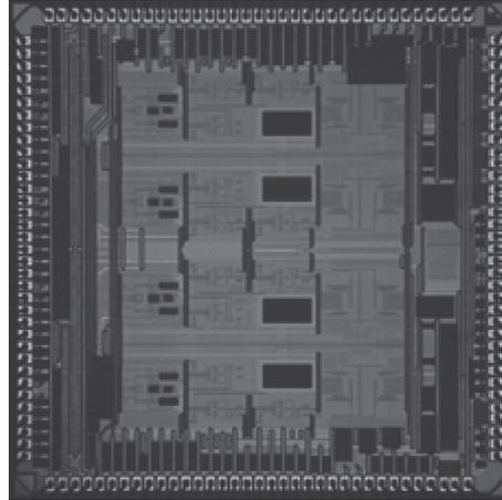
Fig. 3. Chip die of the prototype of custom ADC (NEVIS13) [3]
