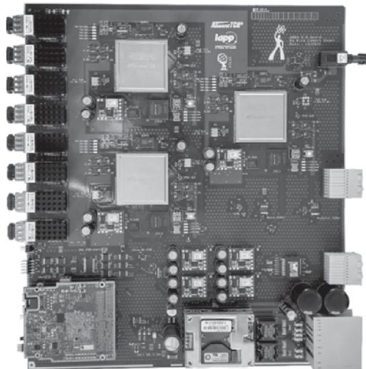
Fig. 7. The pre-prototype LDPB developed in LAPP
