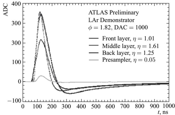
Fig. 12. Responses of four super cells (one from each layer) from LTDB Demonstrator to injected calibration pulses (DAC = 1000 to each LAr cell) [5]
