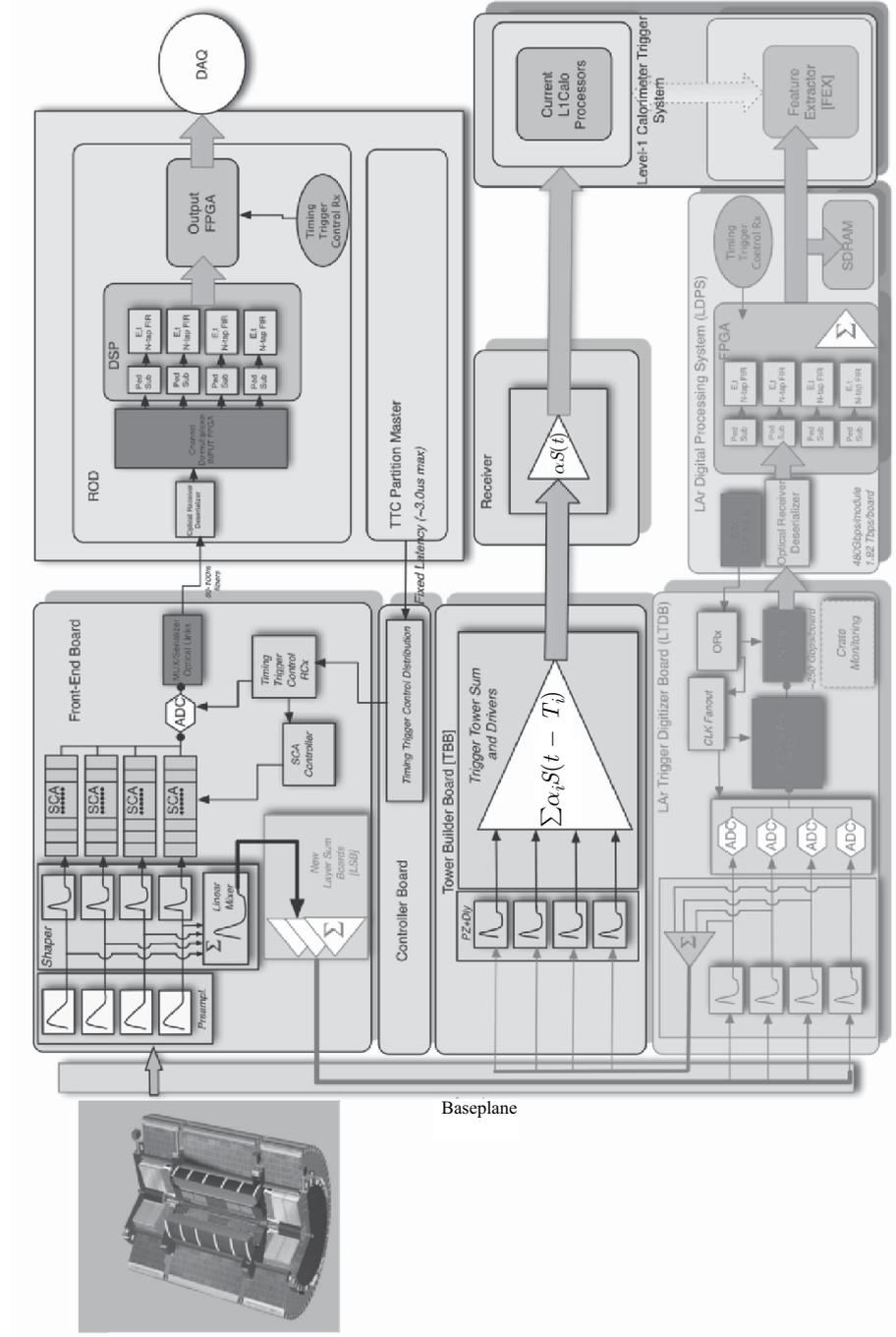
Fig. 2. Schematic diagram of the architecture of the readout electronics after the Phase-I Upgrade
