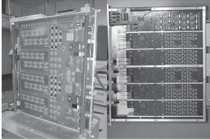
Fig. 6. The two types of LTDB demonstrators, developed by BNL (left) and LAL/Saclay (right), respectively
