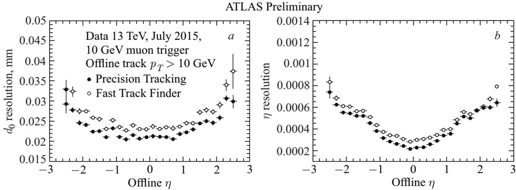
Fig. 5. ID tracking resolution in  $d_0$  (a) and  $\eta$  (b) in muon trigger [10]
