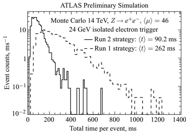
Fig. 1. Improvement from the redesigned ID tracking algorithm in Run 2 [10]
