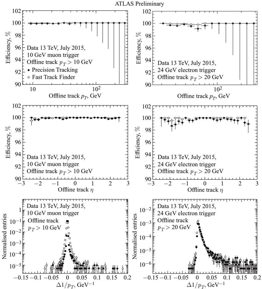
Fig. 4. ID tracking performance in the muon (left) and electron (right) triggers [10]
