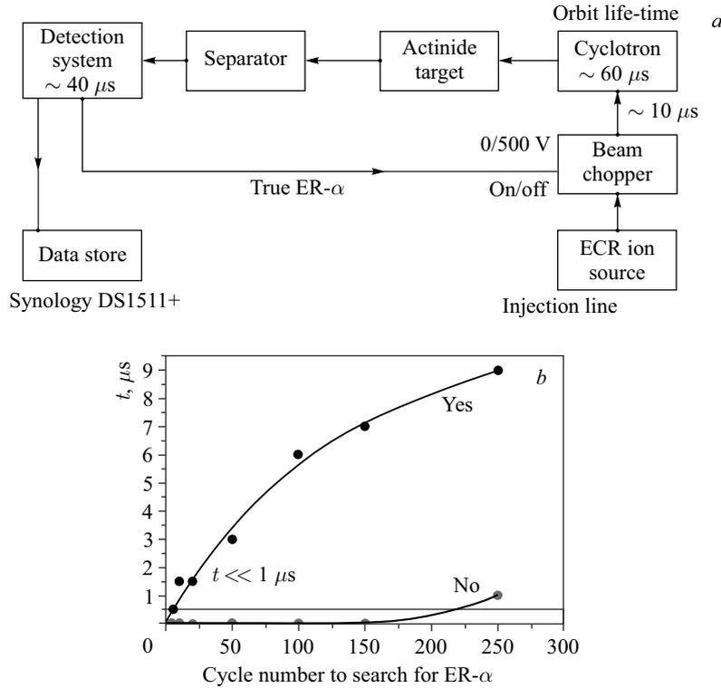
Fig. 1. a) Block diagram of real-time process. Two key elements are shown in yellow. b) Extra time  $t \ll 1 \mu\text{s}$  which is required ( $n = 1$  is actual) to search for ER- $\alpha$  correlation (Yes scenario)
