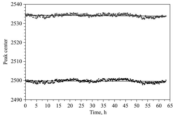
Fig. 6. Tests for the ADP-16 TechInvest module (bottom graph is a 65-h stability test)
