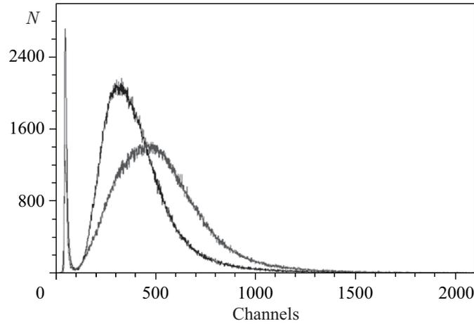
Fig. 5.  $\Delta E$  spectra (channels) measured with the START and STOP low-pressure proportional counters of the DGFRS
