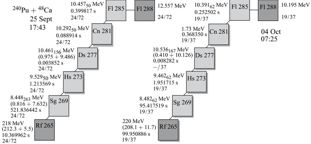
Fig. 3. Two registered sequences of  $Z = 114$  nuclei. (Shadows are beam off phases. See also [6])
