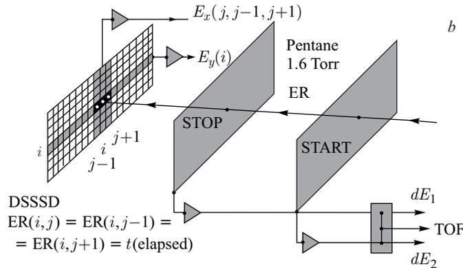
Fig. 2. DSSSD detector of the DGFRS (*a*) and schematics of “beam off” intervals creating (*b*). The formation process for ER matrix is shown in (*b*). Edge effects for neighbor back-side strips are taken into account (for some cases one may apply two neighbor pixels of ER’s matrix except for three ones)
