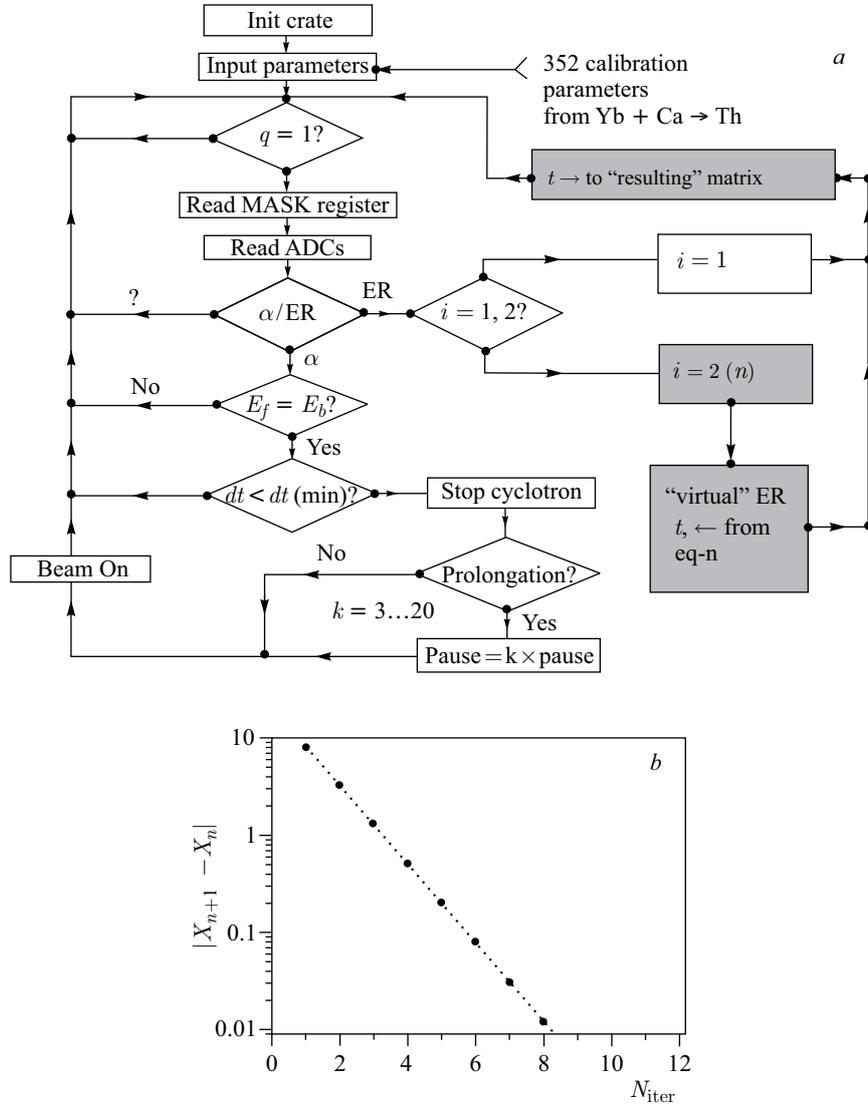
Fig. 4. a) The flowchart of ER- $\alpha$  search process ( $k = 3-20$ ). b) The convergence process for the Newton iteration method. (Y axis is displayed as %, X axis represents number of iterations)
