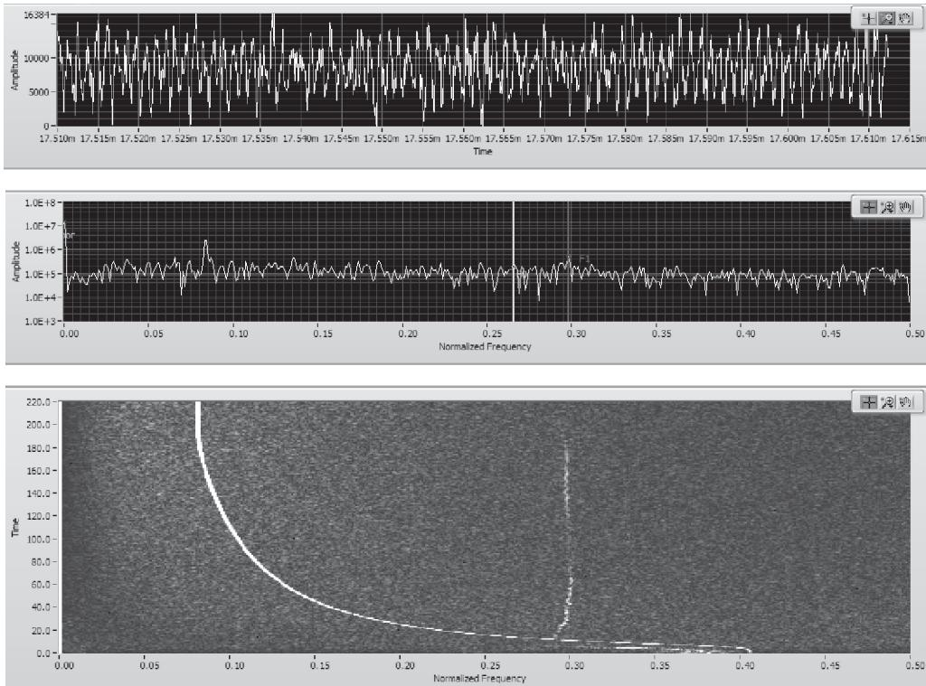
$Q_x$  measurement during acceleration with mixed constant frequency 50 kHz from the signal generator (bright track on the left of the figure), the ADC sampling frequency is equal to the beam revolution frequency, excitation signal is white noise, frame size is 1024 samples, measured value of  $Q_x$  is 0.283
