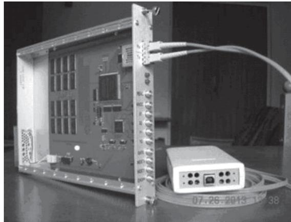
Fig. 1. DeLiDAQ-2D module for data acquisition from PSD
