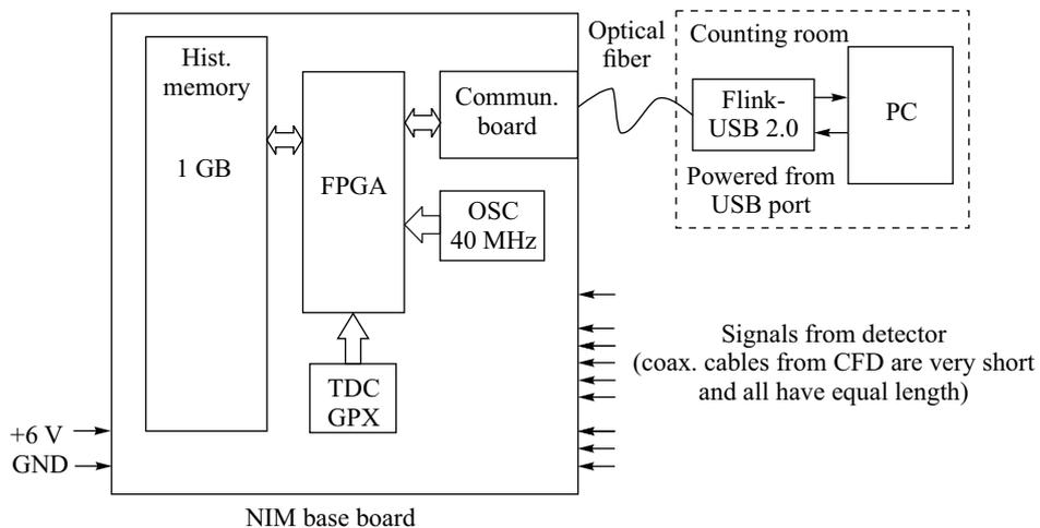
Fig. 2. Architecture of a new system with DeLiDAQ-2D for data acquisition
