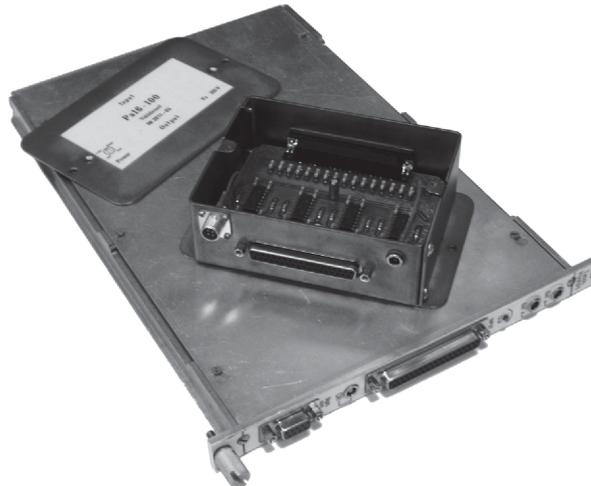
Fig. 2. Multichannel preamplifier and multiplexer-amplifier
