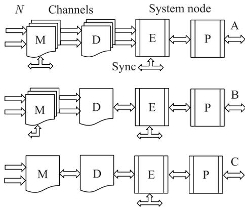
Fig. 1. Procedure flowcharts of A, B and C type. The operations M, D, E and P represent measuring, data acquisition, link exchange and process control
