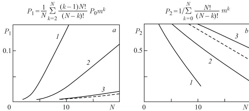
Fig. 2. Coefficients of the idle time  $P_1$  (a) and  $P_2$  (b) at the number  $N$  of channels. Graphs 1, 2 and 3 are shown at the values of the factor  $m$  equal to 0.1, 0.05 and 0.025, respectively
