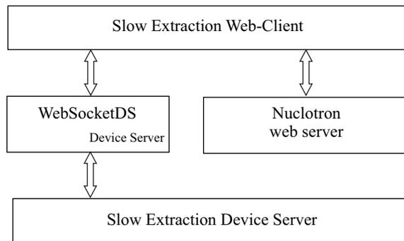
Fig. 5. Interconnection diagram of the Slow Extraction Control Web-Client
