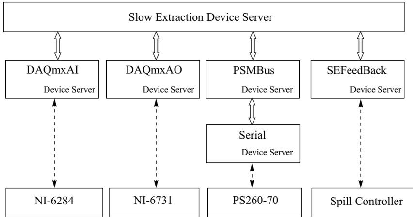
Fig. 3. Diagram of the equipment control by the Slow Extraction Device Server
