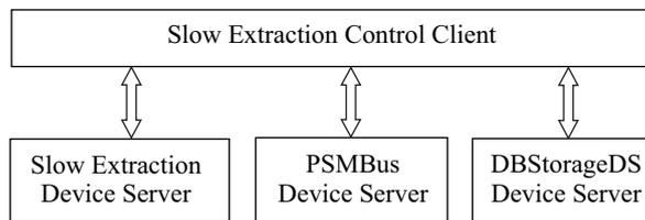
Fig. 4. Interconnection diagram of the Slow Extraction Control Client
