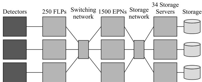
Fig. 2. High-level overview of the data aggregation, from the fragments read-out from the detectors to the full Time Frames stored on the Storage Servers [2]
