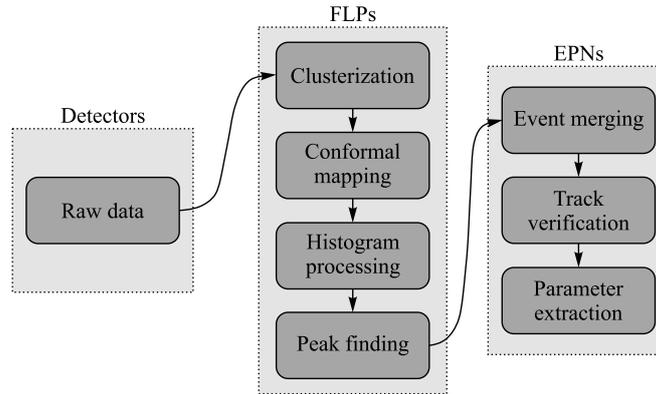
Fig. 4. Overview of the main steps in the HT based reconstruction for the TPC
