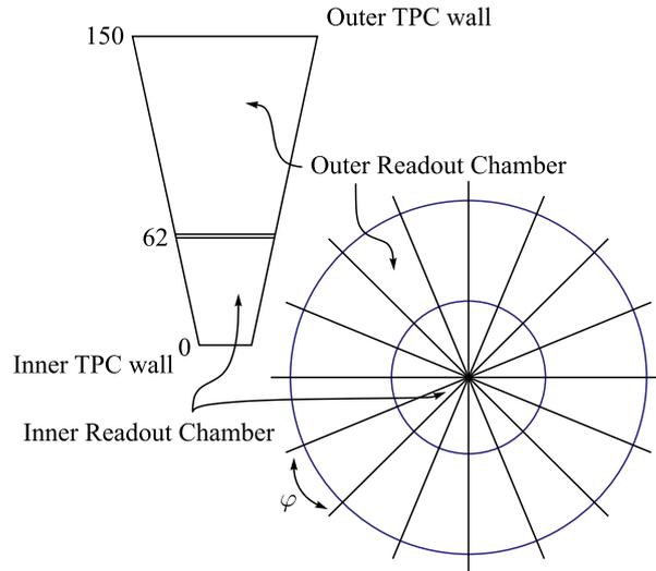
Fig. 1. A schematic view of the current layout of the TPC sectors and readout chambers
