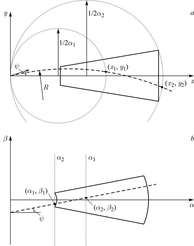
Fig. 3. a) A schematic view of a TPC sector on the Cartesian cluster system. The dashed line represents a track crossing the sector. The two defined circles are also visible. b) The same view in the conformal mapping space. The track and the two circles are visible as straight lines [4]
