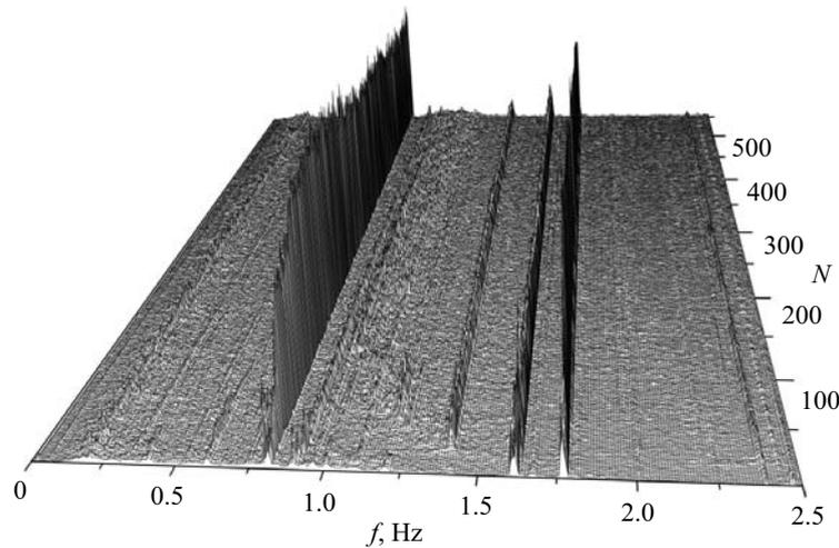
Fig. 2. Variation in the power spectrum of the IBR-2M pulse energy fluctuations during one of the typical reactor operation cycles at the power of 2 MW. The measurement duration is 10.5 days; 552 spectra are presented
