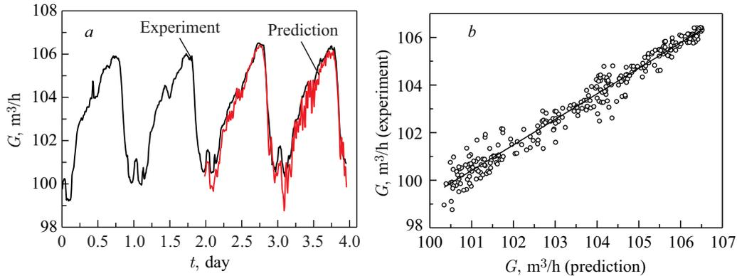
Fig. 4. Comparison between measured daily liquid sodium flow rate through the core of the IBR-2M and predicted one by the proposed model NAR (a). Experimental results versus predicted data (b)
