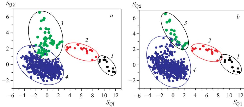
Fig. 3. Cluster structures compressed from the 256-d to the two-d space for the total pulse energy fluctuations (a) and the fluctuations due to the axial vibrations of the moving reflectors (b)
