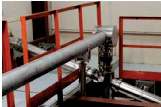
Fig. 4. Optical beamlines for the first and the second stage FELs. Radiation of both FELs is delivered to the same user stations. Switching between FELs is done by retractable mirror
