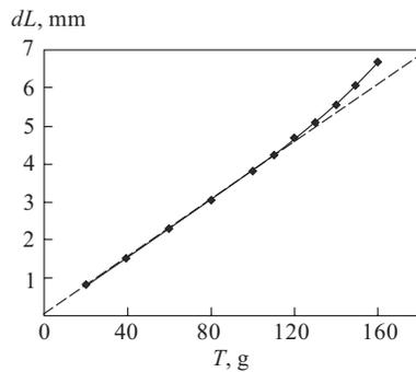
Fig. 6. Dependence of linear lengthening of a 1 m long anode wire on its tension
