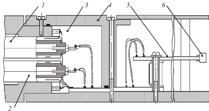
Fig. 3. A scheme of the gas volume and a peripheral part of the chamber: 1, 2 — bottom and top straw-planes; 3 — gas volume; 4 — demountable cover of the gas volume; 5 — readout; 6 — connector used to install a readout map
