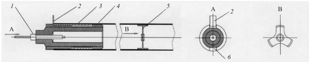
Fig. 7. A scheme of straw (1) with inserted end-plug (2) and spacer (3). Pin (4) for fixing an anode wire, ring spring (5) for grounding the straw cathode, gas channel (6)
