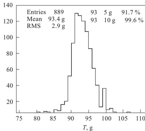
Fig. 8. A typical histogram of wire tension in the chamber
