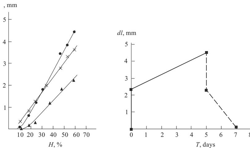
Fig. 10. Lengthening of the 3.2 m long straw depending on air humidity: ● — KK<sub>Loaded-C</sub> straw; × — MK<sub>Loaded-C</sub>; ▲ — 2K<sub>Coated-C</sub>
