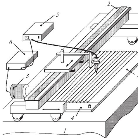
Fig. 5. Kinematics of gluing a fragment of the straw-plane. Precision table (1); linear module (2) with engine (3) used to move a syringe with glue along the straws; precision rulers (4); glue dispenser (5); control block (6)
