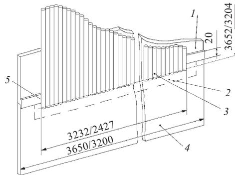
Fig. 2. Glueing the straw-plane with the orthogonal Al rods oriented across the straws: 1 — bottom element of the Al frame made with an accuracy of better than 0.1 mm; 2 — boundary dimensions of the future total gas volume; 3 — straw-plane; 4 — Al element used to place peripheral elements of the chamber; 5 — area of tight strong pasting the straw-plane with the Al element
