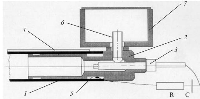
Fig. 9. A scheme of the internal end of straw (1) in an insensitive zone; end-plug (2) with wire-fixing pin (3); fiber glass frame (4) 1 mm in thickness,  $230 \times 220$  mm in size and with an internal hole of  $200 \times 200$  mm; ring groove (5) for hermetic straw sealing and connection of the termination RC chain to the cathode; metal tube (6); gas manifold (7)
