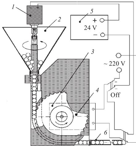
Fig. 4. Kinematics of filling the straw with precision balls. The mixer with engine (1) and volume (2) containing precision balls; pushing gear (3) with engine (4); power unit (5); straw (6)
