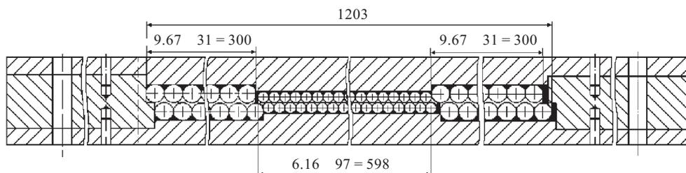
Fig. 1. Cross section of the ST2 detectors prototype
