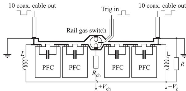
Fig. 3. Scheme of high-voltage generator
