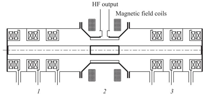
Fig. 1. Schematic of a driver with a magnetron
