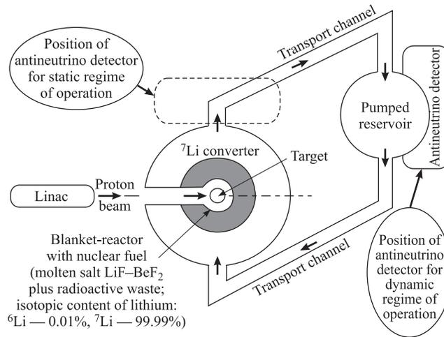
Fig. 3. Scheme of the lithium antineutrino source on the basis of the booster-type neutron source. Variants for the static and dynamic regimes of operation
