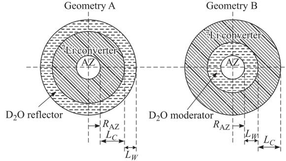
Fig. 2. Geometry of the multilayer converter
