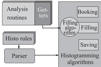
Flow chart of the generic data analysis. The histogramming is separated from the analysis. The algorithm is defined in metafiles, the parser generates the C++ code for histogram booking, filling and storing
