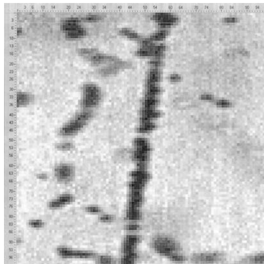
Fig. 4. View of the particle track in the nuclear photoemulsion layer at fixed z coordinate, detected by means of the confocal scanning microscope SOLAR TII
