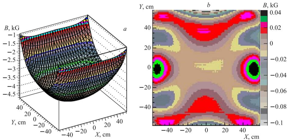
Fig. 3. The most significant magnetic field component  $B_y$  in the detector station after the first iron absorber ( $z = 125$  cm) calculated using polynomial approximation (a) and the difference between the approximation and the field map (b)
