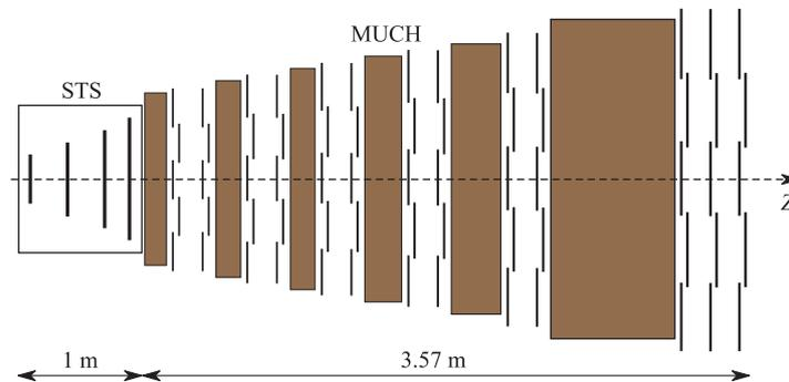
Fig. 1. Sketch of the silicon tracking system (STS) and the muon detector (MUCH)
