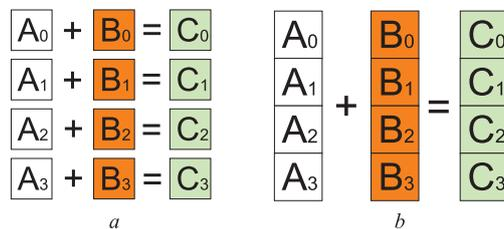
Fig. 2. Comparison between scalar (*a*) and SIMD (*b*) summation. With scalar summation four add instructions are executed one after another, meanwhile, SIMD uses only one add instruction to achieve the same result
