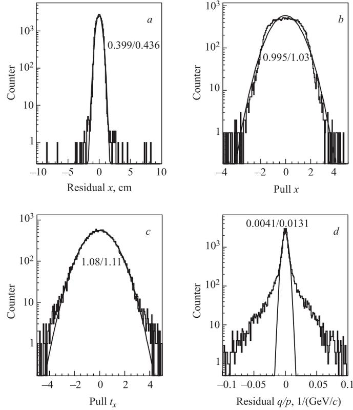
Fig. 4. Selected performance distributions for the SIMDized track fitter algorithm at the last MUCH station: a)  $x$  residual; b)  $x$  pull; c)  $t_x$  pull; d)  $q/p$  residual. Numbers show the width of a Gaussian fitted to the distributions (first number) and the root mean square value as second number
