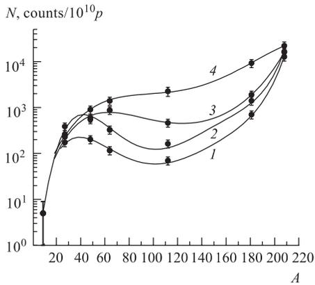
Fig. 4.  $A$ -dependence of the number of counts for the assembly T-D-T and four energies of incident protons 0.3 (1), 0.6 (2), 1.0 (3) and 2.2 GeV (4). The points — experimental results; the curves — result of fitting
