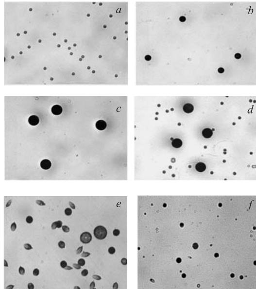
Fig. 1. Detector's surface with etched tracks; *a*)  $^{16}\text{O}$  ions (20 keV/ $\mu\text{m}$ ); *b*)  $^{40}\text{Ar}$  ions (92 keV/ $\mu\text{m}$ ); *c*)  $^{56}\text{Fe}$  ions (402 keV/ $\mu\text{m}$ ); *d*) blind 1 (mixture of Fe and O) from ICCHIBAN 8; *e*)  $^{252}\text{Cf}$  fission fragments; *f*) proton induced tracks of secondary particles — plateau region
