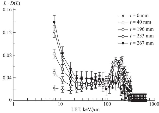
Fig. 4.  $L \cdot D(L)$  distributions for different depth in water and 205 MeV proton beam, normalized at each depth to the dose due to particles with LET above  $7 \text{ keV}/\mu\text{m}$
