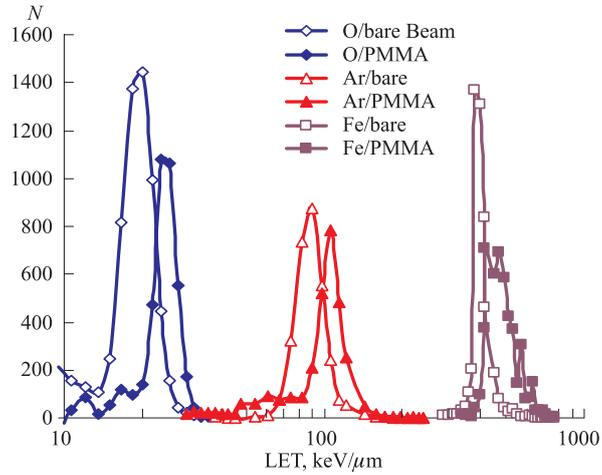
Fig. 8. LET spectra of various ions ( $^{16}\text{O}$ ,  $^{40}\text{Ar}$ ,  $^{56}\text{Fe}$ ) in Page PADTable 1. Relative contribution to the dose from primary  $^{12}\text{C}$  ions (480 MeV/amu)
