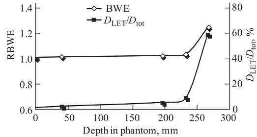
Fig. 5.  $D_{\text{rel}} = D_L/D_{\text{tot}}$  and RBWE in 205 MeV proton beam as a function of residual proton energy
