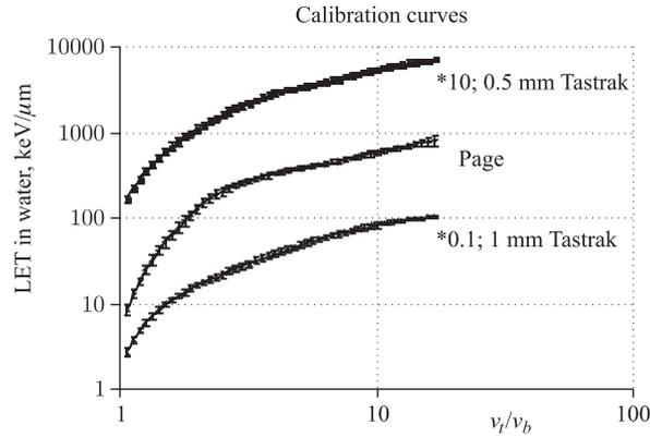
Fig. 2. Calibration curves for PADCs
