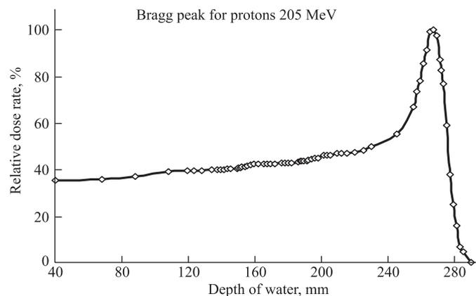
Fig. 3. Relative depth–dose distribution in 205 MeV proton beam measured with thin Si detector
