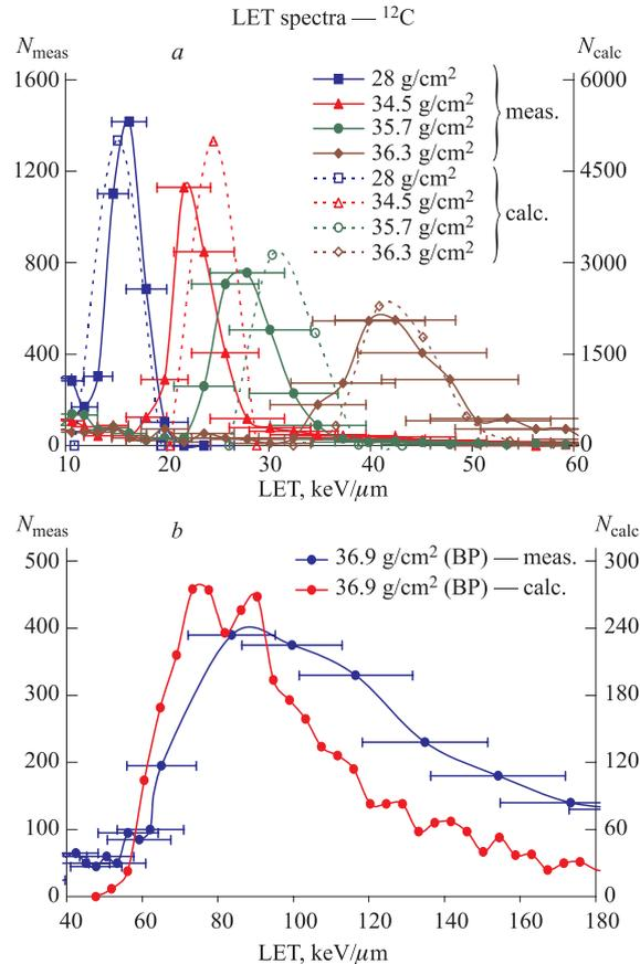
Fig. 6. Track number distributions in LET measured with LET spectrometer and calculated with SRIM code
