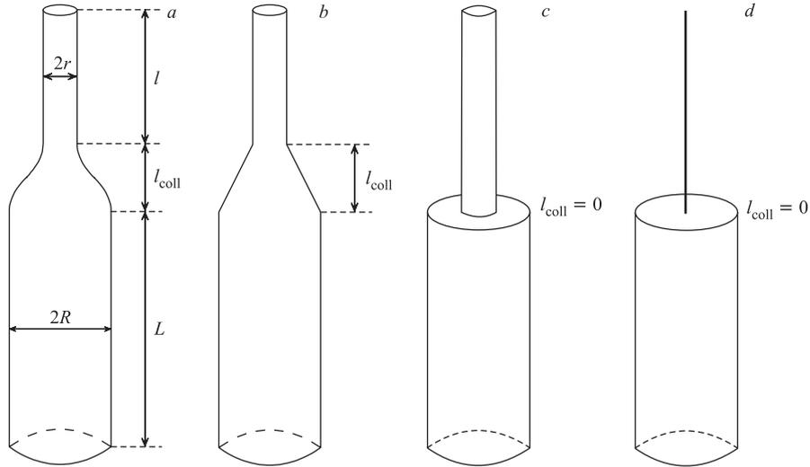
Fig. 1. *a*) Wine bottle with a long body and a long neck; *b*) bottle with a conical collar; *c*) bottle with a horizontal collar; *d*) bottle with a horizontal collar and a thread-like neck
