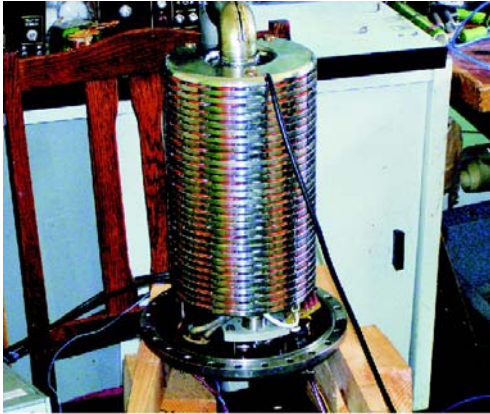
Fig. 3. High-voltage generator assembly
