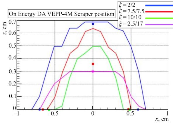
Fig. 4. The results of simulation with experimental points
