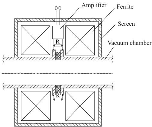
Fig. 2. Design of the symmetric monitor
