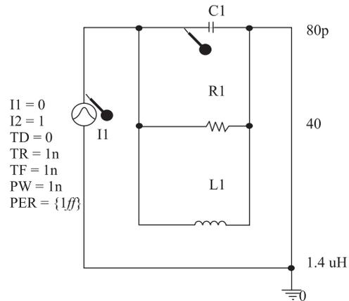
Fig. 3. The equivalent circuit of the detector
