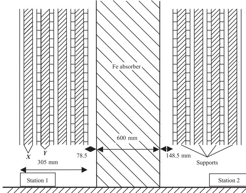
Fig. 1. Schematic side view of the MW1 detector
