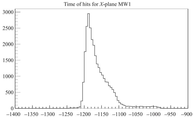
Fig. 8. Drift time spectrum: the scale is in ns
