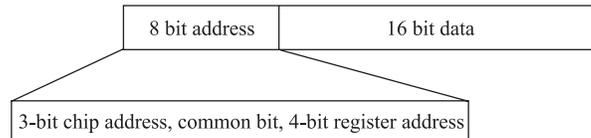
Fig. 4. Structure of the setup data format
