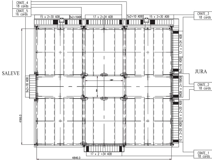
Fig. 2. Front view of one of the MW1 stations. The positions of the front-end boards are shown together with the euro-crates housing the digital cards
