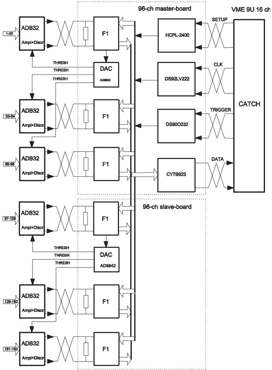
Fig. 3. Block diagram of the digital card
