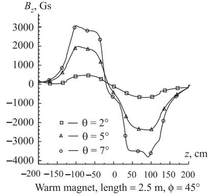
Fig. 18. The behavior of  $B_z$  field component along rays in polar coordinate system for  $\varphi = 45^\circ$
