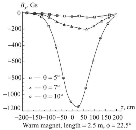
Fig. 15. The behavior of the  $B_x$  field component along rays in the polar coordinate system for  $\varphi = 22.5^\circ$
