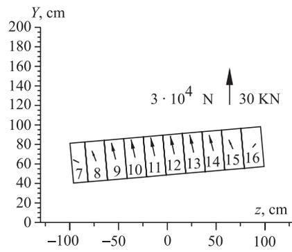
Fig. 23. Side view of the coil and force components  $jF_y + kF_z$
