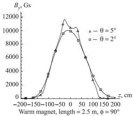
Fig. 14. The behavior of the main field component along rays in the polar coordinate system for  $\varphi = 90^\circ$
