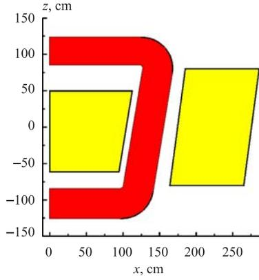
Fig. 6. The magnet cross section by the plane  $y = 0.7$  m for  $x \geq 0$
