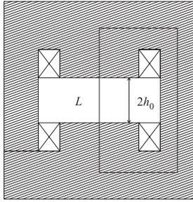
Fig. 2. Cross section of a magnet with coil placement of the first type
