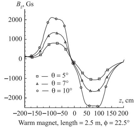
Fig. 17. The behavior of the  $B_z$  field component along rays in the polar coordinate system for  $\varphi = 22.5^\circ$
