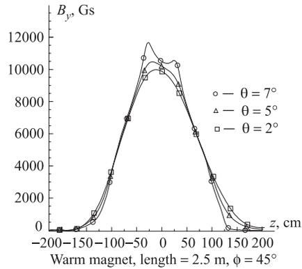
Fig. 13. The behavior of the main field component along rays in the polar coordinate system for  $\varphi = 45^\circ$
