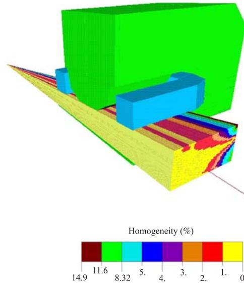
Fig. 19. Distribution of bending power homogeneity in the working region
