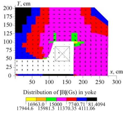
Fig. 8. Distribution of  $|\mathbf{B}|$  in yoke and field behavior for plane  $z = 0$  and  $x, y \geq 0$
