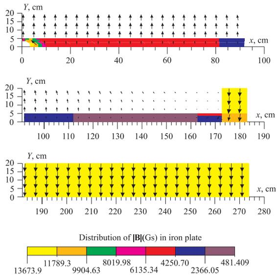
Fig. 20. Distribution of  $|B|$  in the iron plate and field behavior for plane  $z = 0$  and  $x, y > 0$
