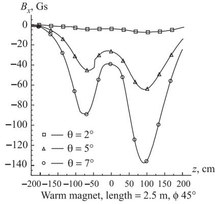
Fig. 16. The behavior of the  $B_x$  field component along rays in the polar coordinate system for  $\varphi = 45^\circ$
