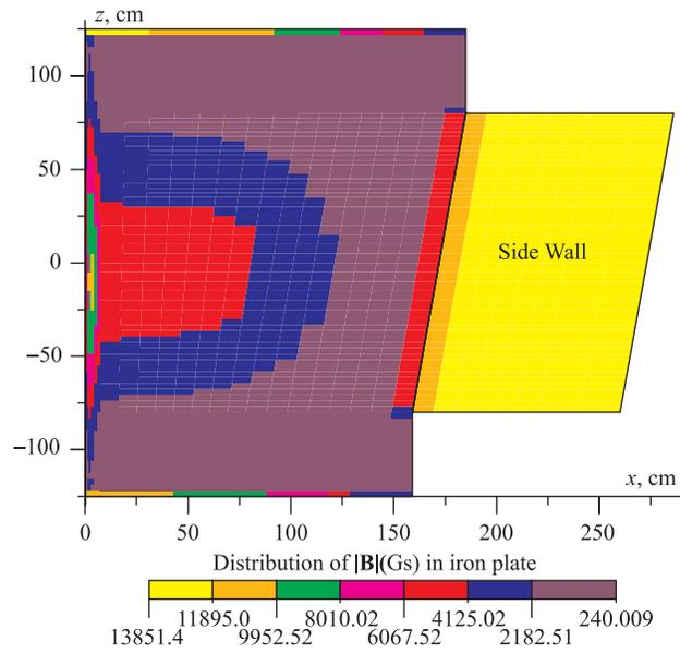
Fig. 21. Distribution of  $|B|$  in the iron plate for plane  $y = 4.125$  cm and  $x \geq 0$
