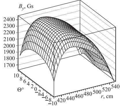
Fig. 7. The coil field in working region for plane  $y = 0$
