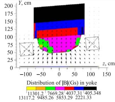
Fig. 9. Distribution of  $|\mathbf{B}|$  in yoke and field behavior for plane  $x = 0$  cm and  $y \geq 0$
