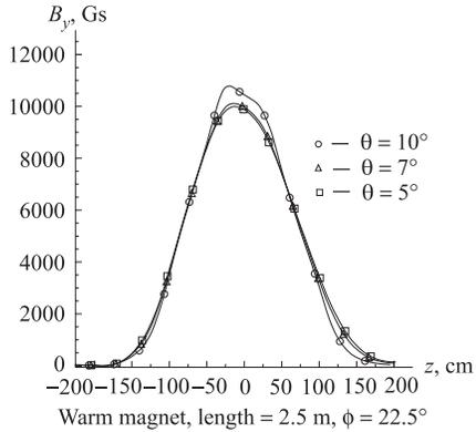
Fig. 12. The behavior of the main field component along rays in the polar coordinate system for  $\varphi = 22.5^\circ$
