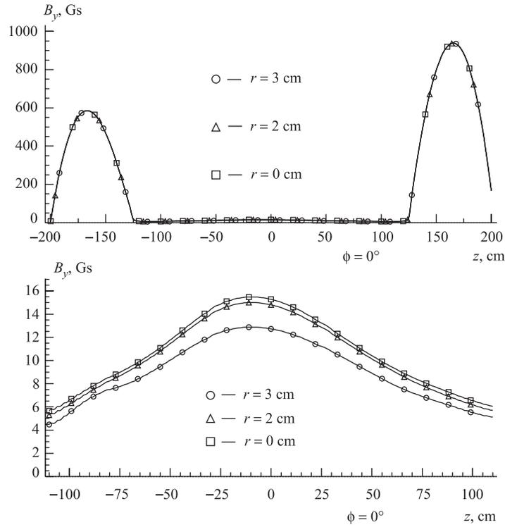
Fig. 11. The behavior of the main field component in the channel (polar coordinate system),  $\varphi = 0^\circ$
