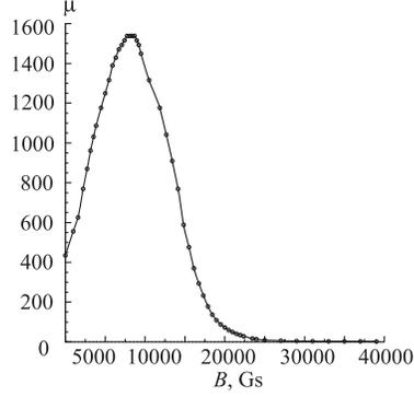
Fig. 4. The magnetic characteristic  $\mu(|\mathbf{B}|)$  for steel 3
