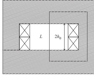
Fig. 3. Cross section of a magnet with coil placement of the second type
