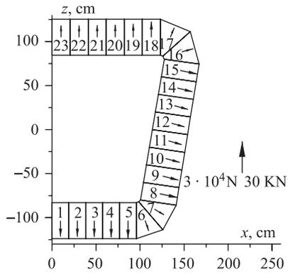
Fig. 22. Top view of the coil and force components  $iF_x + kF_z$
