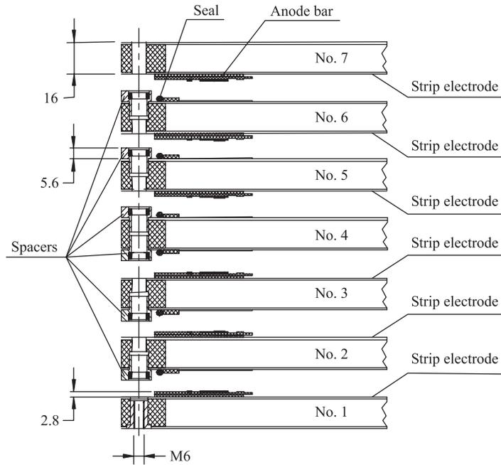
Fig. 1. P3 cross-section
