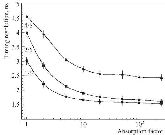
Fig. 6. CSC timing resolution for different majority coincidence options as a function of the absorption factor
