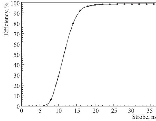
Fig. 5. CSC registration efficiency vs. strobe width for 4/6 majority scheme
