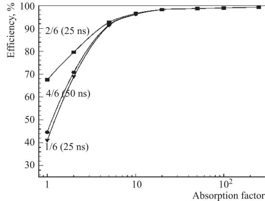
Fig. 7. The CSC efficiency vs. absorption factor for 25- and 50-ns strobe widths
