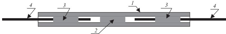
Fig. 1. Glass capillary tube (1) for the electrically separate connection of two anodes (4). Central isolation part (2), zone of the wire solder (3)
