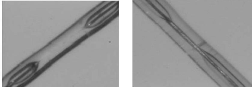
Fig. 3. Fragments of the capillary tube. The central isolation part (left) and zone of the wire solder inside the tube (right)
