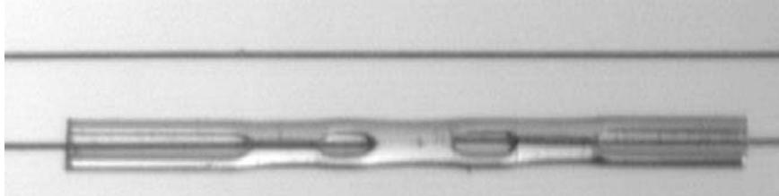
Fig. 2. Wire-joint by the glass tube contains two soldered wires inside the tube. Diameter of the wire is 30  $\mu\text{m}$ . The similar wire is stretched above the joint to show its straightness
