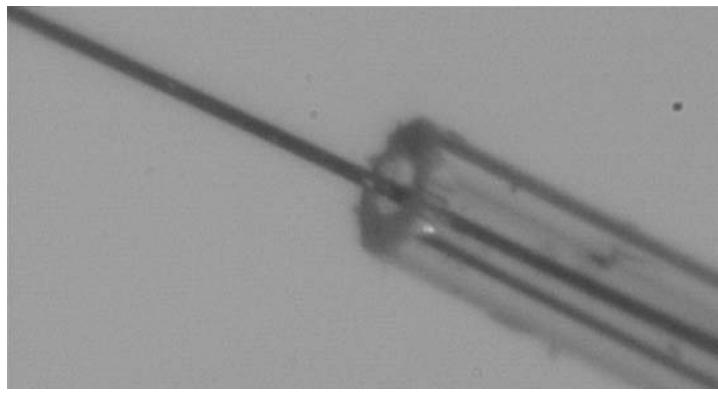
Fig. 4. End face of the capillary tube with the soldered anode wire
