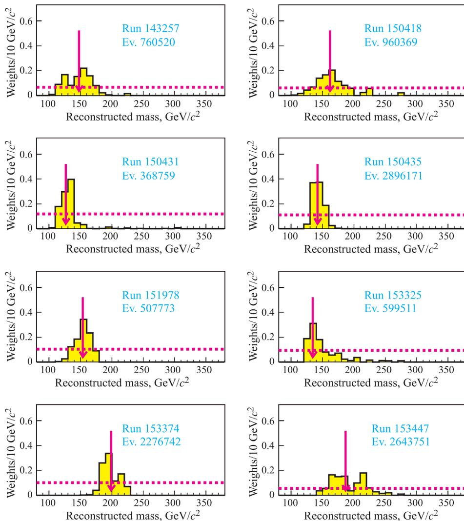
Fig. 1. Binned weight (probability) distributions for first 8 data events. The red arrow corresponds to the estimated top mass of the event. The dashed line shows our cut (30% of maximum)
