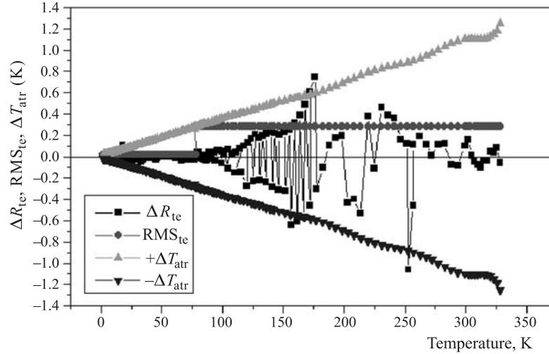
Fig. 5. Temperature dependences of the deviations  $(\Delta R)_{te}$ ,  $RMS_{te}^R$  and  $\pm\Delta T_{atr}$  for three-interval approximation of CERNOX–RuO<sub>2</sub> composition thermometer
