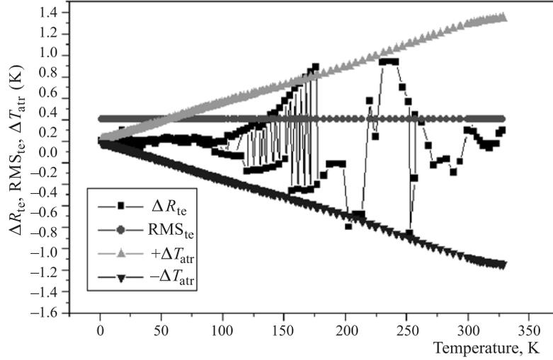
Fig. 4. Temperature dependences of the deviations  $(\Delta R)_{te}$ ,  $RMS_{te}^R$  and  $\pm\Delta T_{atr}$  for the whole interval approximation of CERNOX–RuO<sub>2</sub> composition thermometer
