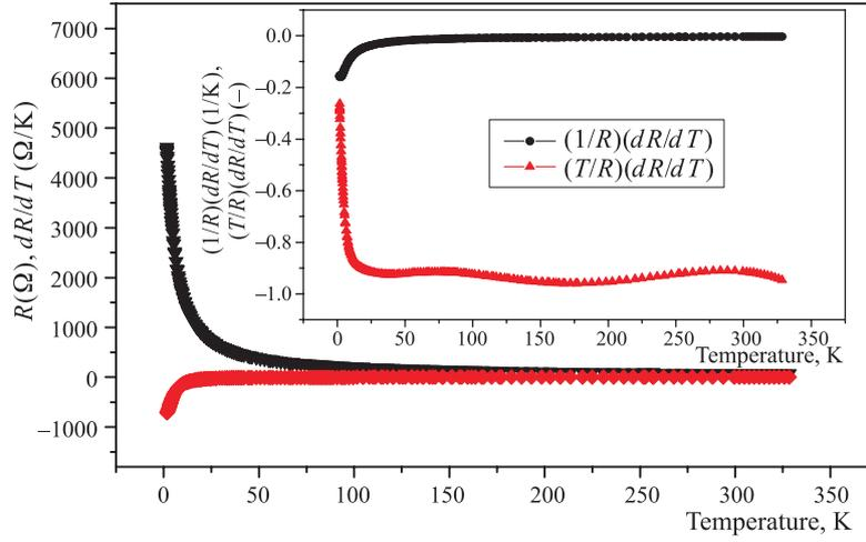
Fig. 1. Temperature dependences of the resistance  $R$ , the absolute  $dR/dT$ , relative  $1/R(dR/dT)$  and specific  $(T/R)(dR/dT)$  sensitivities for the whole interval approximation of CERNOX–RuO<sub>2</sub> composition thermometer
