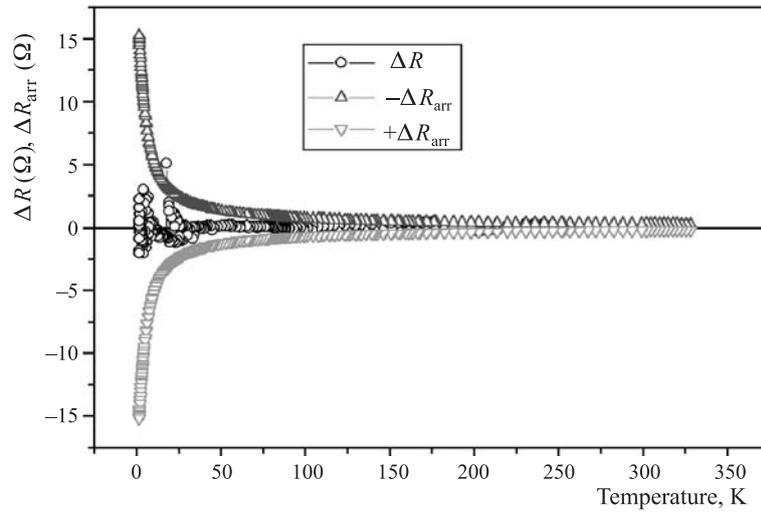
Fig. 3. Temperature dependences of the resistance deviations  $\Delta R$  and  $\pm\Delta R_{arr}$  for the whole interval approximation of CERNOX–RuO<sub>2</sub> composition thermometer
