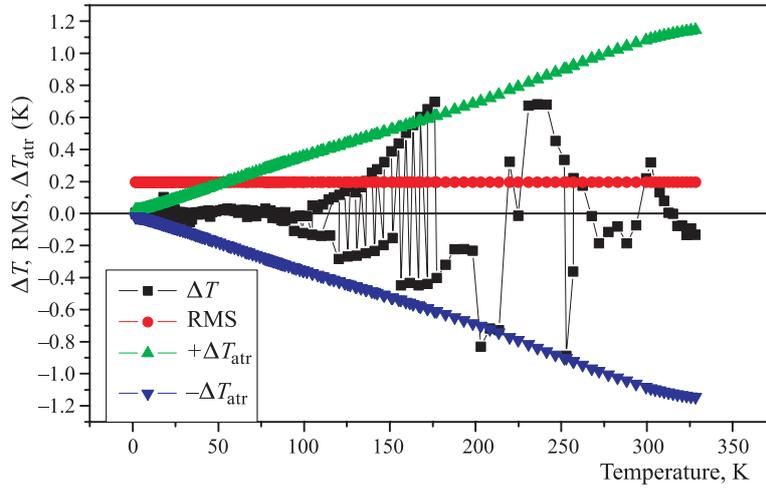
Fig. 2. Temperature dependences of the deviations  $\Delta T$ ,  $RMS^T$  and  $\pm\Delta T_{atr}$  for the whole interval approximation of CERNOX–RuO<sub>2</sub> composition thermometer
