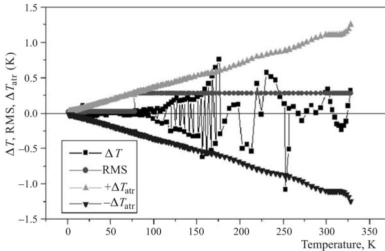
Fig. 6. Temperature dependences of the deviations  $\Delta T$ ,  $\text{RMS}^T$  and  $\pm\Delta T_{\text{atr}}$  for three-interval approximation of CERNOX–RuO<sub>2</sub> composition thermometer
